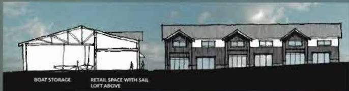
BOAT STORAGE RETAIL SPACE WITH SAIL LOFT ABOVE SAIL BOAT STORAGE AND RETAIL SECTION AND NORTH ELEVATION 1" = 20' - 0"
